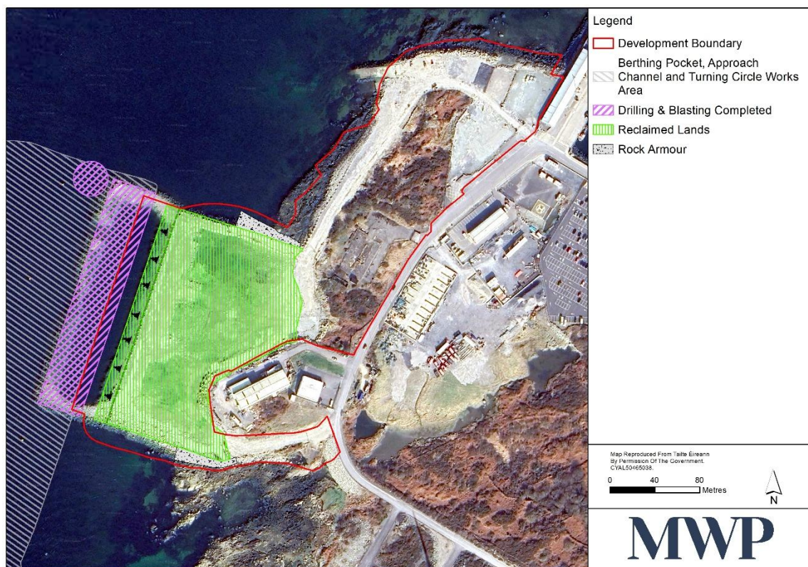
Figure 4: Map indicating the development works area, including the reclamation area, the blasting and dredging areas, the berm construction areas and rock armour placed undertaken between Jan 2023 and May 2024
